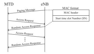
Fig. 3. System signaling procedures of the contention resolution-based LTE group paging.
