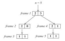
Fig. 2. Example of the contention resolution scheme with n = 5 MTDs. The number in each slot denotes the number of MTDs involving the contention. If this number is larger than 1 (a collision), then a new frame is assigned to those MTDs. If this number is 0 (an empty slot) or 1 (a successful transmission), the expansion stops.
